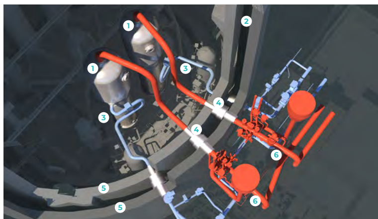
1 Steam generators 2 Annulus 3 Feedwater Flow Control System 4 Penetrations 5 Double containment 6 Steam System (VVP)
