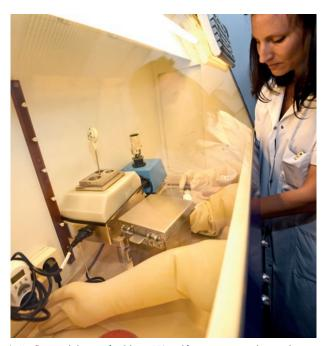
Handling a sealed source of gadolinium-153 used for activity meter quality controls. ASN inspection of Clémentville clinic, Montpellier, May 2017.
