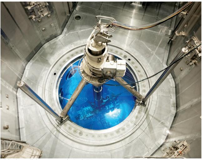
Checks on the EPR vessel by the in-service inspection machine, September 2017.
