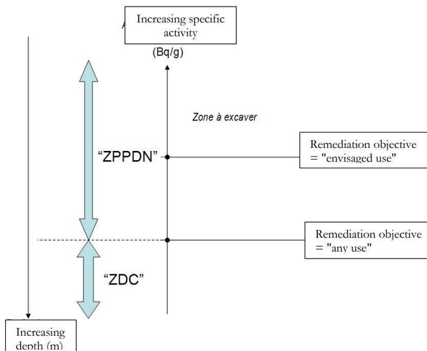
Figure 4: Correspondence between the waste zoning applied to the soil and the remediation objectives
