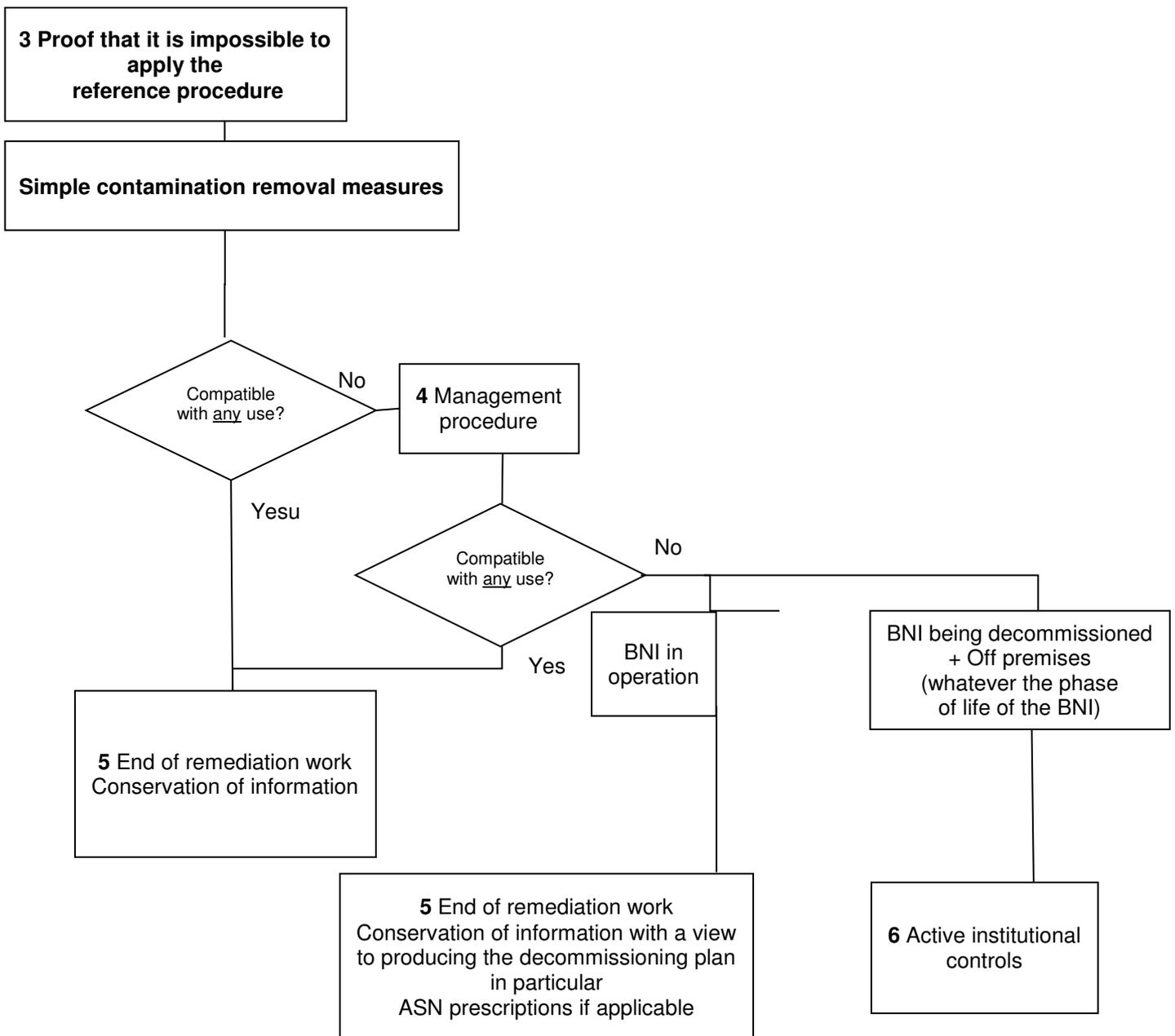
Figure 3: Logic diagram illustrating the steps in the soil management procedure in a BNI
