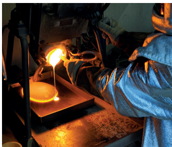
PRODUCTION OF GLASS FOR THE HIGH-LEVEL WASTE VITRIFICATION PROCESS
