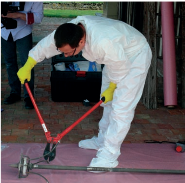
Cutting off the head of a radium lightning arrester
