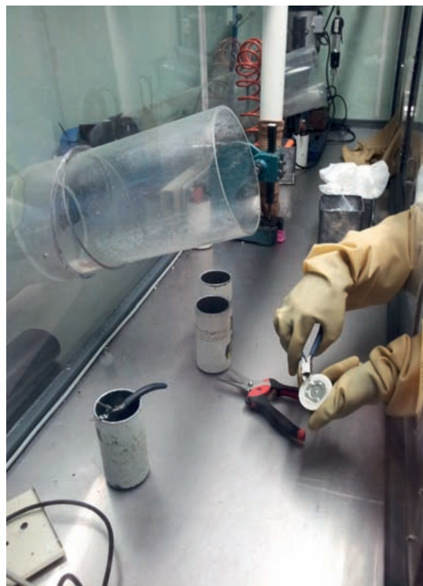
Dismantling of smoke detectors
