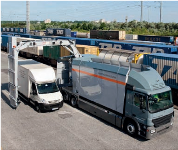
Mobile linear accelerator used for inspecting loads
