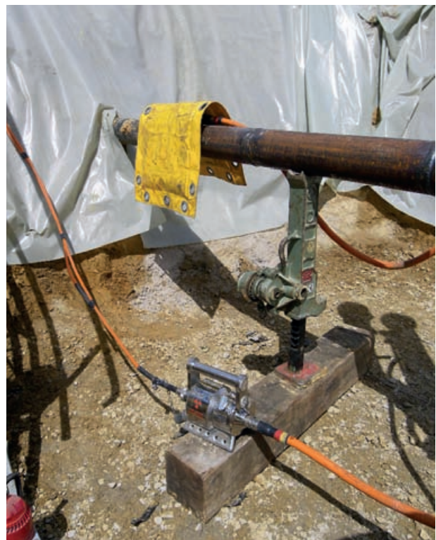
Gamma radiography device on work site
