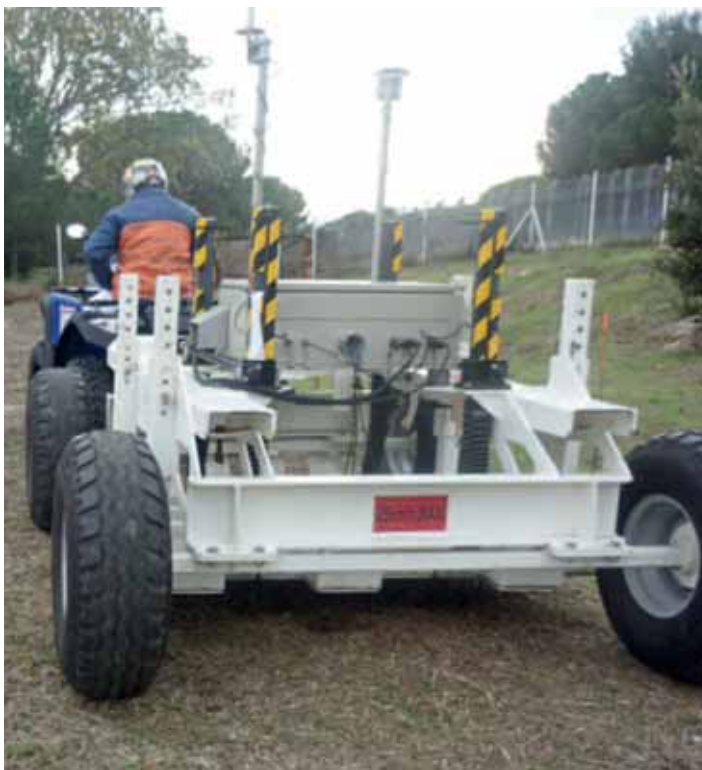
All-terrain radiological inspection system (CRTT)
